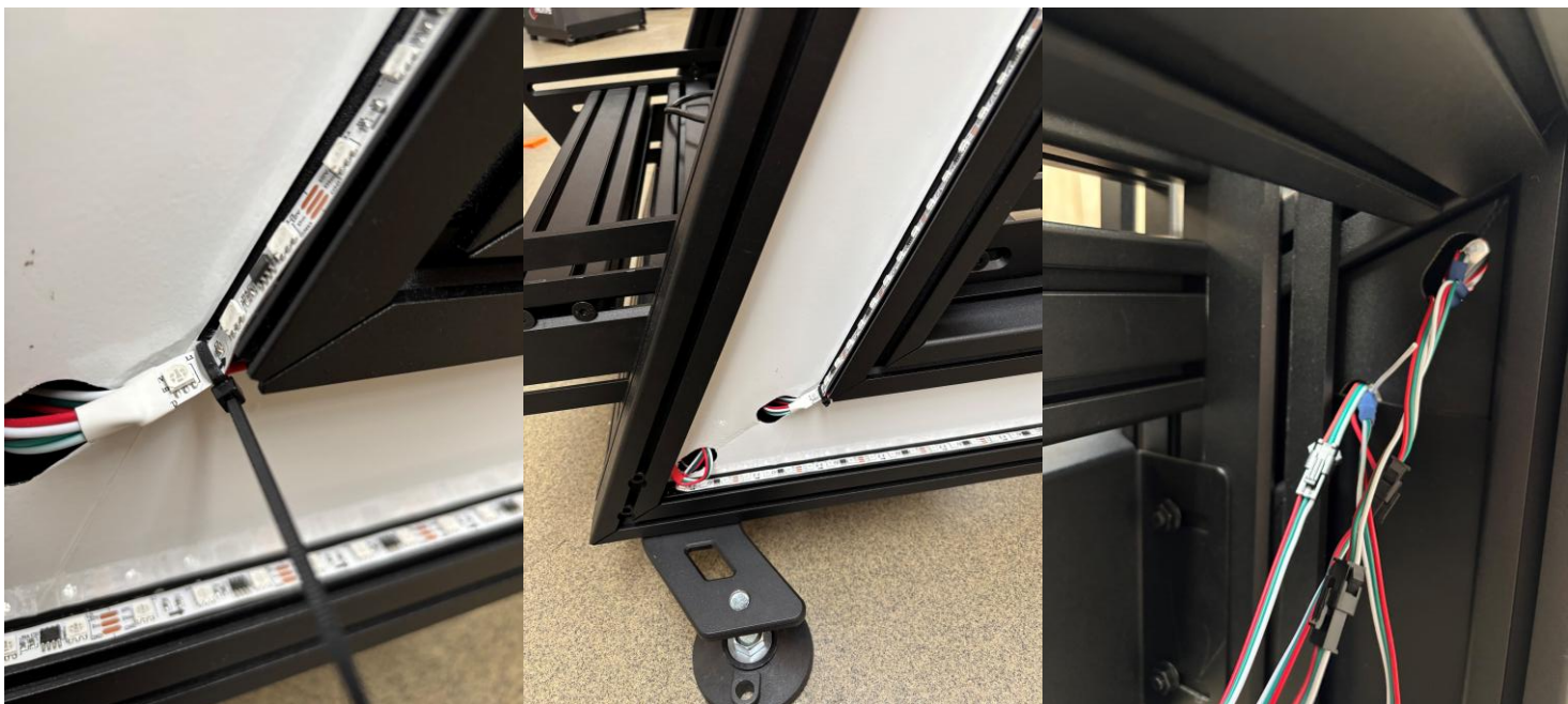
Fasten the cable tie gently
