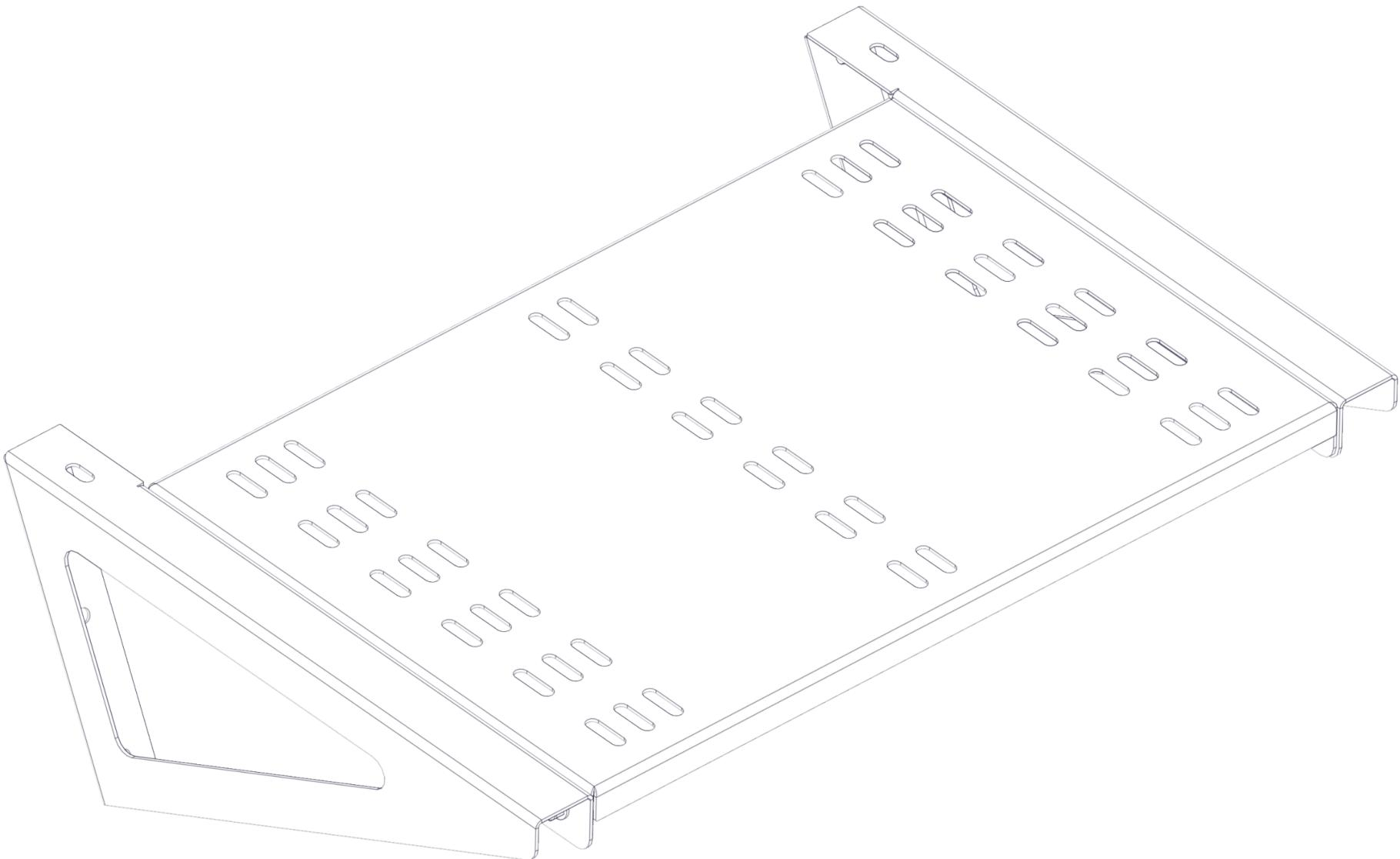
Install the undertray using four C4 M8 nuts and four C5 M8 x 12 screws.
